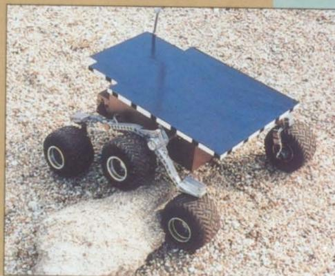
The Mars Surveyor Trolley, named Sojourner, is carried on-board *Mars Pathfinder*, an unmanned spacecraft launched in December. Sojourner, a free-roving probe the size of a child's wagon, will photograph the Martian surface and determine the composition of rocks on Mars.
